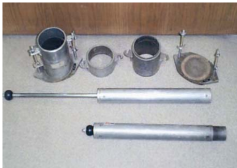
Equipment for the Proctor test, resulting in a diagram of the OMC versus the dry unit weight.
