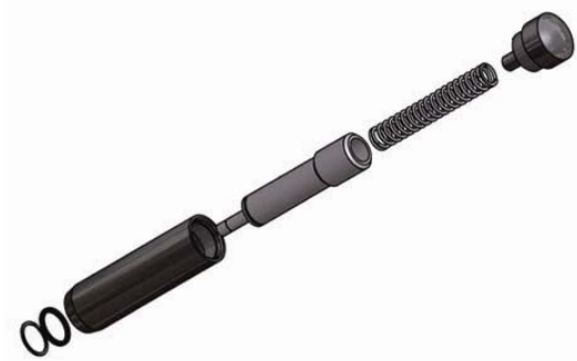
Test the compression of freshly made blocks with the penetrometer.
